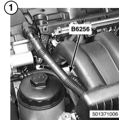
B6256 Dual temperature sensor (coolant tem- perature)
